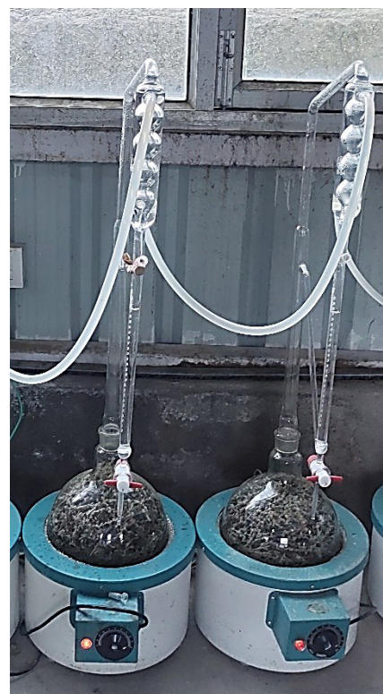
Essential oil extraction of Clary sage var. 'Him Sage' through hydrodistillation
